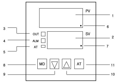
1) Displays processing value(PV) : Displays processing value in controlling and each kind of parameters in parameter set
